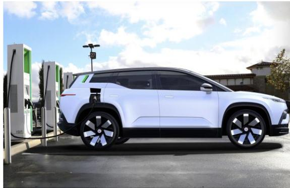
*The Fisker Ocean at an Electrify America charging station. The high mounted side indicators double as charge indicators – signaling a full battery when the green light bar is lit to the top.*
